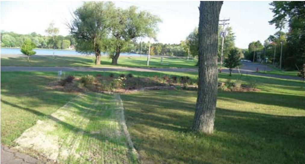
A **rain garden** collects runoff from a parking area and alley. It **prevents** pollutants on the pavement from entering North Twin lake.
